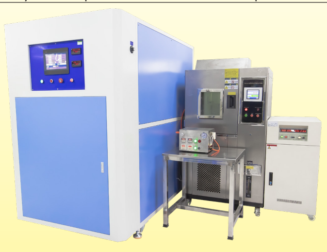
Electrical life test equipment for air switches. (Used for verification of compliance with applicable UL and CE standards)
