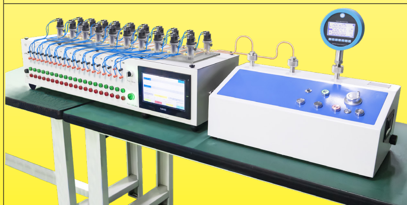
Verification of pressure switch calibration
