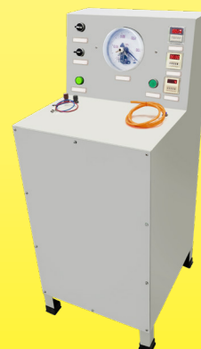
Checking air switch operating cycles
